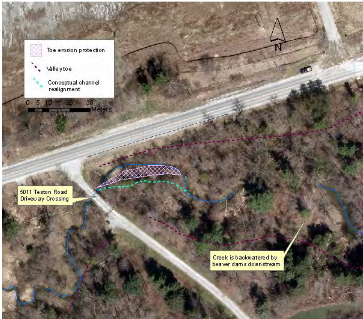
FIGURE 8c Road Embankment Option 3: Road Widening to the South, Proposed Toe Erosion Protection, and Channel Realignment
