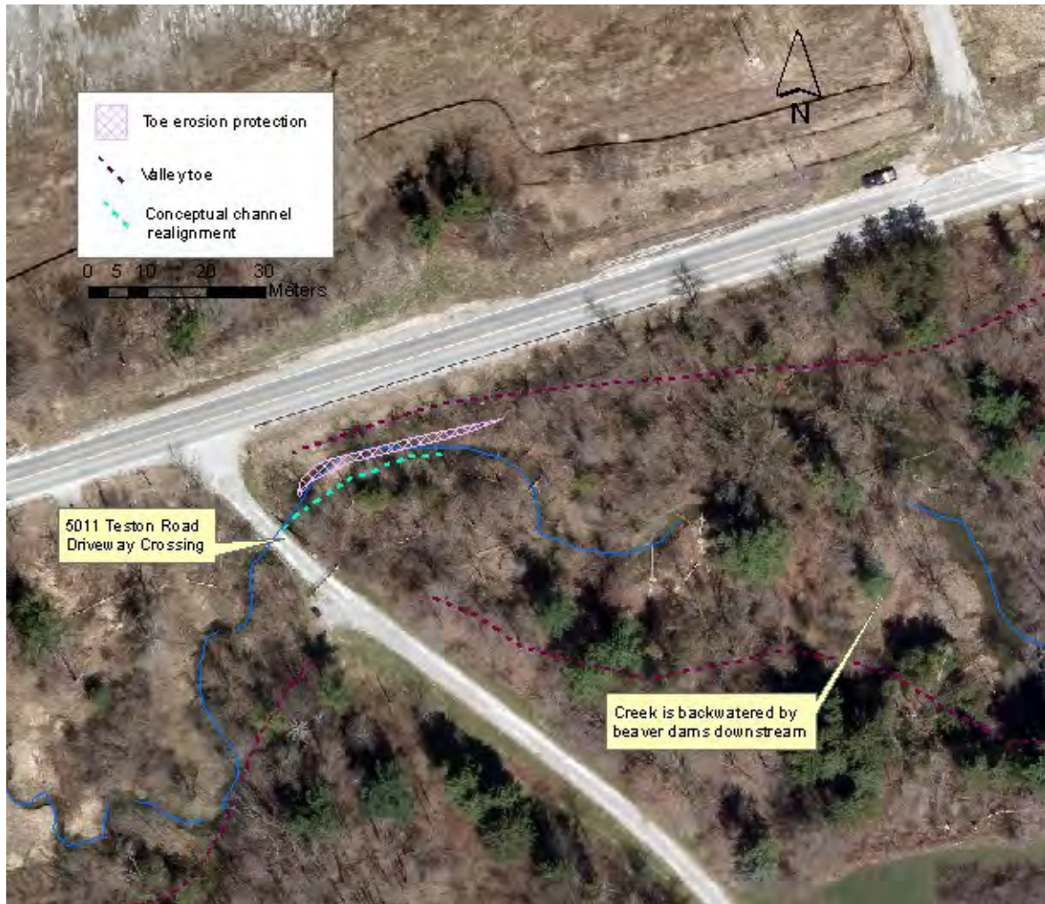
FIGURE 8b Road Embankment Option 2: Road Widening Along Existing Centreline, Proposed Toe Erosion Protection, and Channel Realignment
