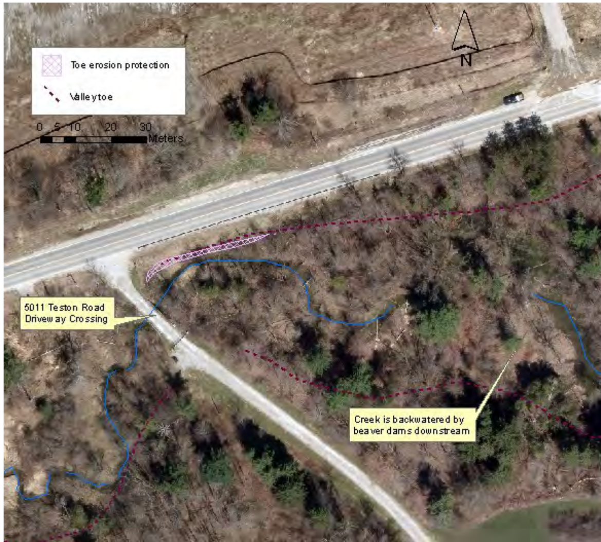
FIGURE 8a Road Embankment Option 1: Road Widening to the North, Proposed Toe Erosion
