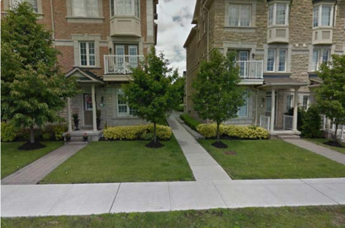
The separation between townhouse blocks should be 3 to 6 metres and be landscaped. (Guideline 5.9)
