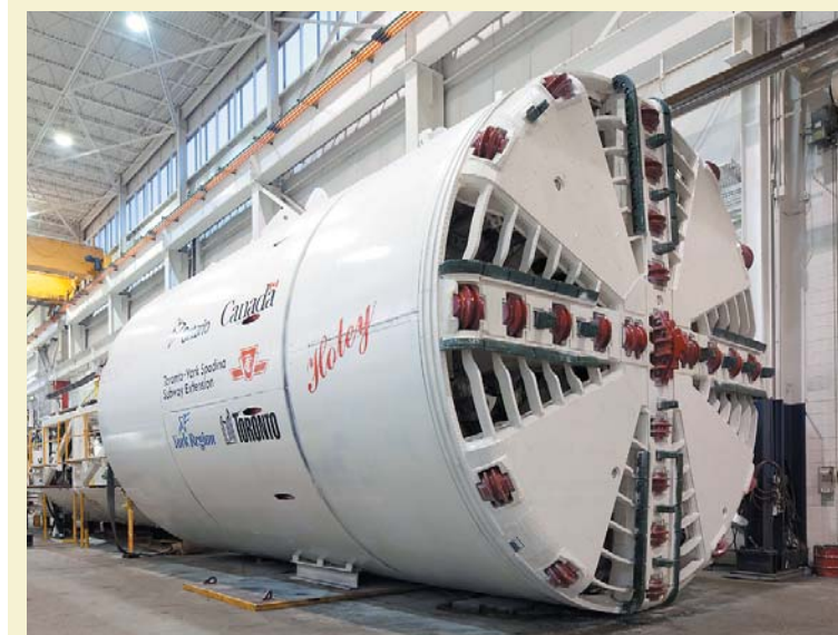
Tunnel Boring Machine "Holey"
